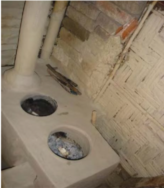
BCSIR 2 pot fixed cookstove with chimney
